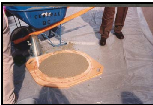
Slump Flow Test
